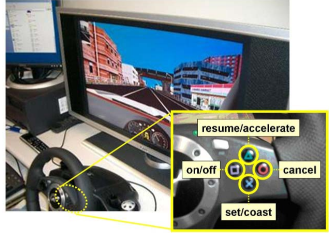
Fig. 1. The driving simulator and the button controllers to manipulate the ACC system.
